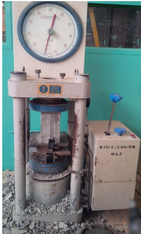
Fig. 1. Stress-strain experimental set-up.
