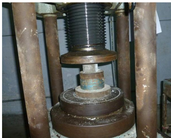
Fig. 2 Cube specimen in testing machine
